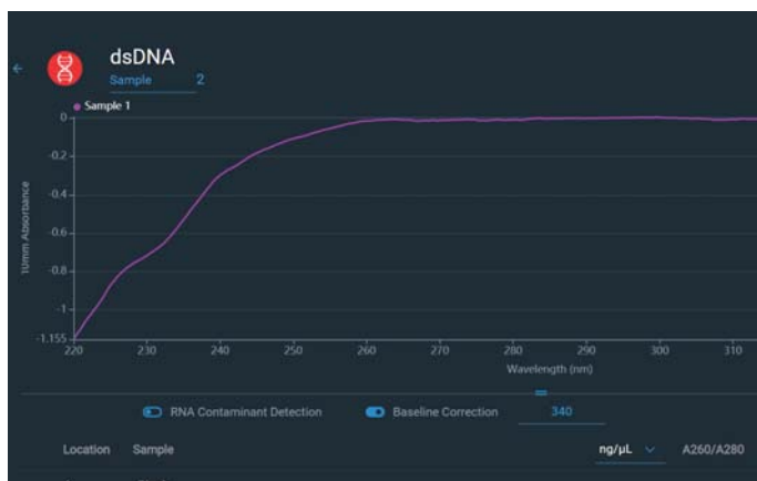
Solution containing salt used to blank instrument results in "mirror image" spectrum
